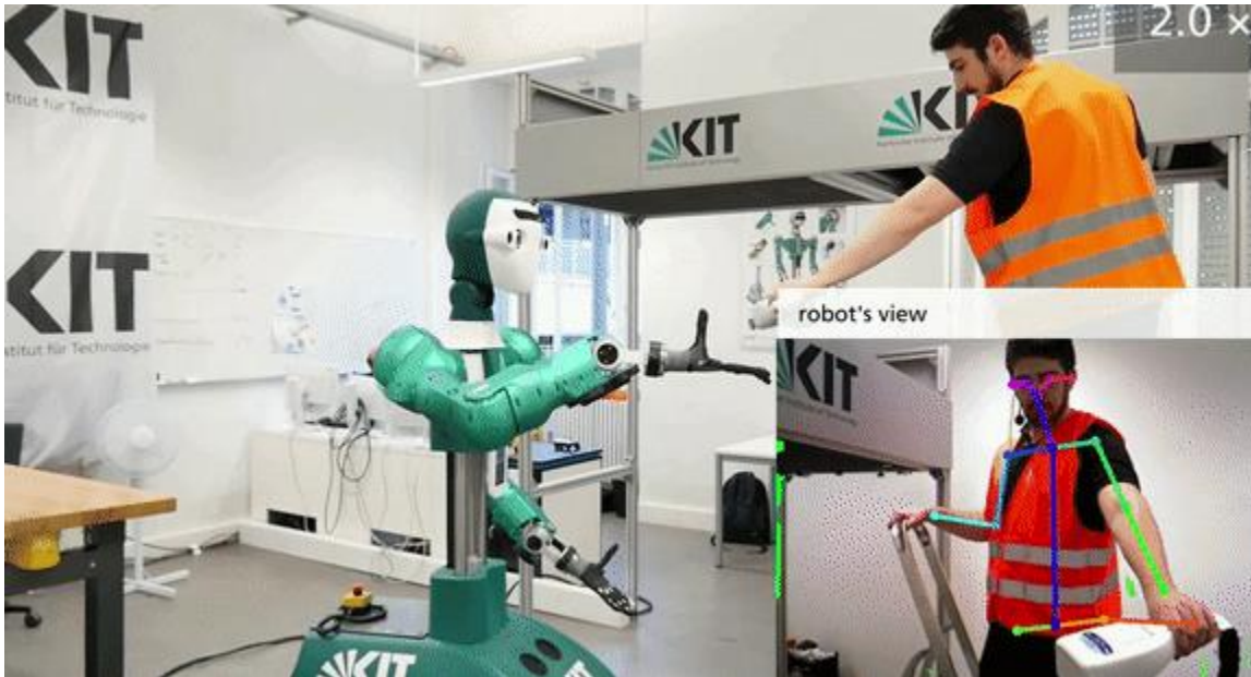
ARMAR-6 using real-time visual data for pose estimation
