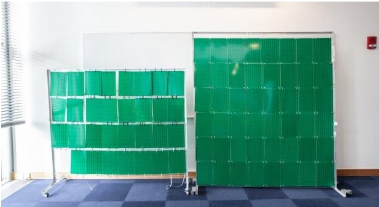
The RFocus platform has more than 3,000 tiny, inexpensive antennas that are used to amplify nearby wireless signals.
