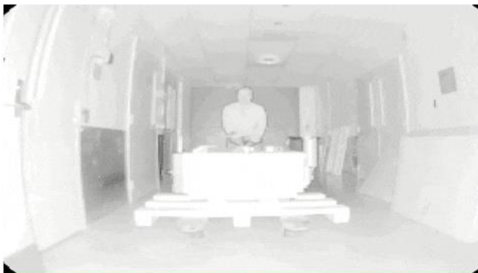
A lidar intensity image of a forklift. Source: Sense Photonics
